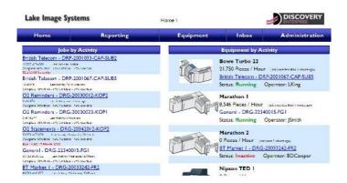
Discovery Enterprise is controlled via it's independent http front end. This allows any PC on the network to access information on any job or equipment to which their user have been given access.
